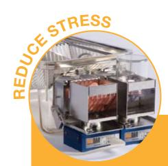
Specially modified plastic shoe box style home cages reduce stress on the animal. The cages provide a suitable environment for long term studies and shorten the acclimation period. Gated hoppers mount outside the cage limiting variability caused by the interaction between researchers and animals.
