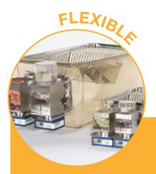
The same electronic components can be used for food or water and for rats or mice allowing a single set to accommodate variable experimental designs. You can choose to run FOOD alone, FOOD + WATER, FOOD + FOOD or WATER + WATER configurations.
